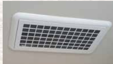
Another feature that we've taken from residential construction is our super quiet "HP" (High performance) 15,000 BTU air conditioning system, which includes a larger compressor and cold air returns! This means 30% more air is being forced into the coach than a standard 15,000 BTU air conditioner.
