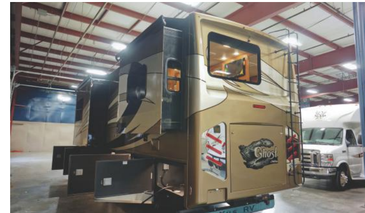
Front to back exterior basement storage with galvanized steel compartments.
