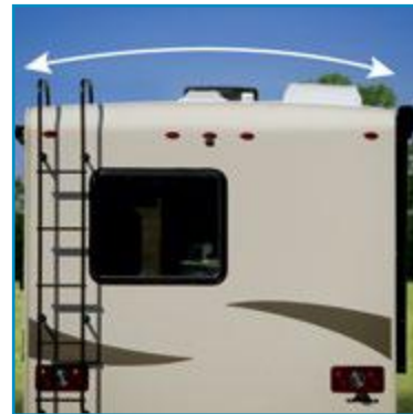
TPO Crowned Roof for Easy Water Runoff
