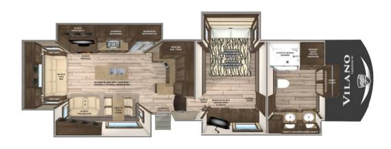
GVWR 16,000 Dry Weight 14,000\* Cargo Carrying 2,000 Width 101" Height 12' 11" \*\* Length 38' 11" \*\*\* Fresh Water Cap. 70 gal Grey Water Cap. 90gal Black Water Cap. 45gal Water Heater 10gal Furnace 42K BTU LP Cap. 60lbs Hitch Weight: 3100\*\*\*\*
