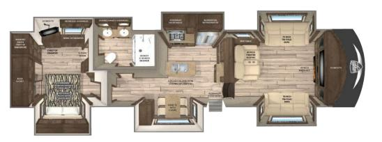
GVWR 16,500 Dry Weight 14,800\* Cargo Carrying 1,700 Width 101" Height 12' 11" \*\* Length 40′ 6″ \*\*\* Fresh Water Cap. 54 gal Grey Water Cap. 90 gal Black Water Cap. 45 gal Water Heater 10 gal Furnace 42K BTU LP Cap. 60 lbs Hitch Weight 3,300\*\*\*\*
