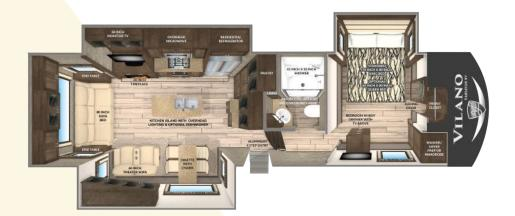
GVWR 16,000 Dry Weight 12,400\* Cargo Carrying 3,600 Width 101" Height 12' 11" \*\* Length 34' 11" \*\*\* Fresh Water Cap. 70 gal Grey Water Cap. 90 gal Black Water Cap. 45 gal Water Heater 10 gal Furnace 42K BTU LP Cap. 60 lbs Hitch Weight 2,600\*\*\*
