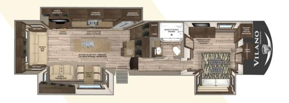
GVWR 16,000 Dry Weight 13,800\* Cargo Carrying 2,200 Width 101" Height 12' 11" \*\* Length 39' 11" \*\*\* Fresh Water Cap. 70 gal Grey Water Cap. 90 gal Black Water Cap. 45 gal Water Heater 10 gal Furnace 42K BTU LP Cap. 60 lbs Hitch Weight 2,800\*\*\*\*
