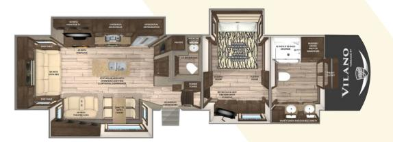
GVWR 16,000 Dry Weight 14,100\* Cargo Carrying 1,900 Width 101" Height 12' 11" \*\* Length 38' 11" \*\*\* Fresh Water Cap. 70 gal Grey Water Cap. 90gal Black Water Cap. 45gal Water Heater 10gal Furnace 42K BTU LP Cap. 60lbs Hitch Weight: 3100\*\*\*\*
