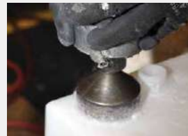
Holding tank fittings are spin-welded for water-tight connections
