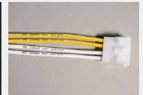
Wiring labeled and spliced to automotive standards
